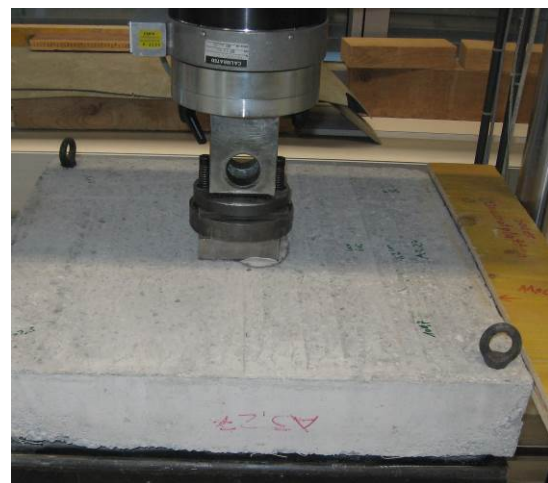
Figure 1 Crack production in interrupted EFNARC square panel test. Test was stopped at a deformation of 3 mm.
