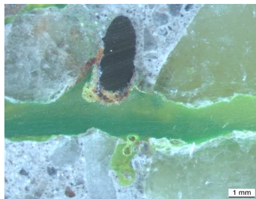
Figure 9 Micrograph of steel fiber near cracks (impregnated for conservation with green resin) at a distance of 35 mm from surface after 1 year exposure in \text{Na}_2\text{SO}_4 -solution (A1).
