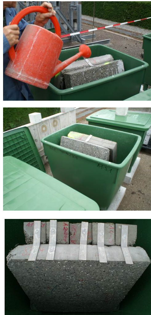
Figure 2 Exposure set-up with application of liquid solutions (top), coverage (center) and different specimens (square panels for mechanical testing and prisms for microscopy, bottom).
